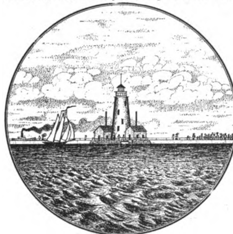
LIGHTHOUSE AND TARGET. Sketch of Telescopic Field, Showing Water Visible at Bottom of Target and Base of Tower.
